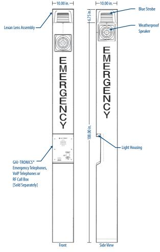
Each Model 234SBA Stanchion Broadcast Assembly is shipped in kit form for field installation. Components included with each complete stanchion assembly are as listed below.
